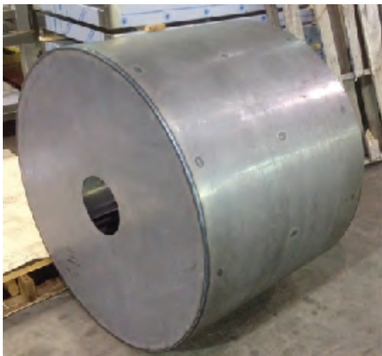
Figure 2 Rear view of the drum with the hole for the atomizer
