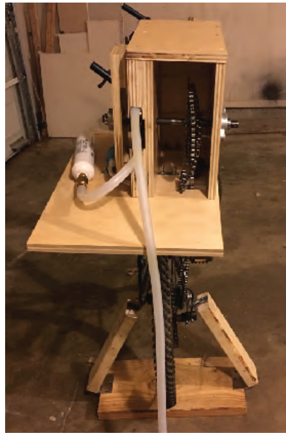
Figure 2 shows the finished peristaltic pump, designed and built by the team.
