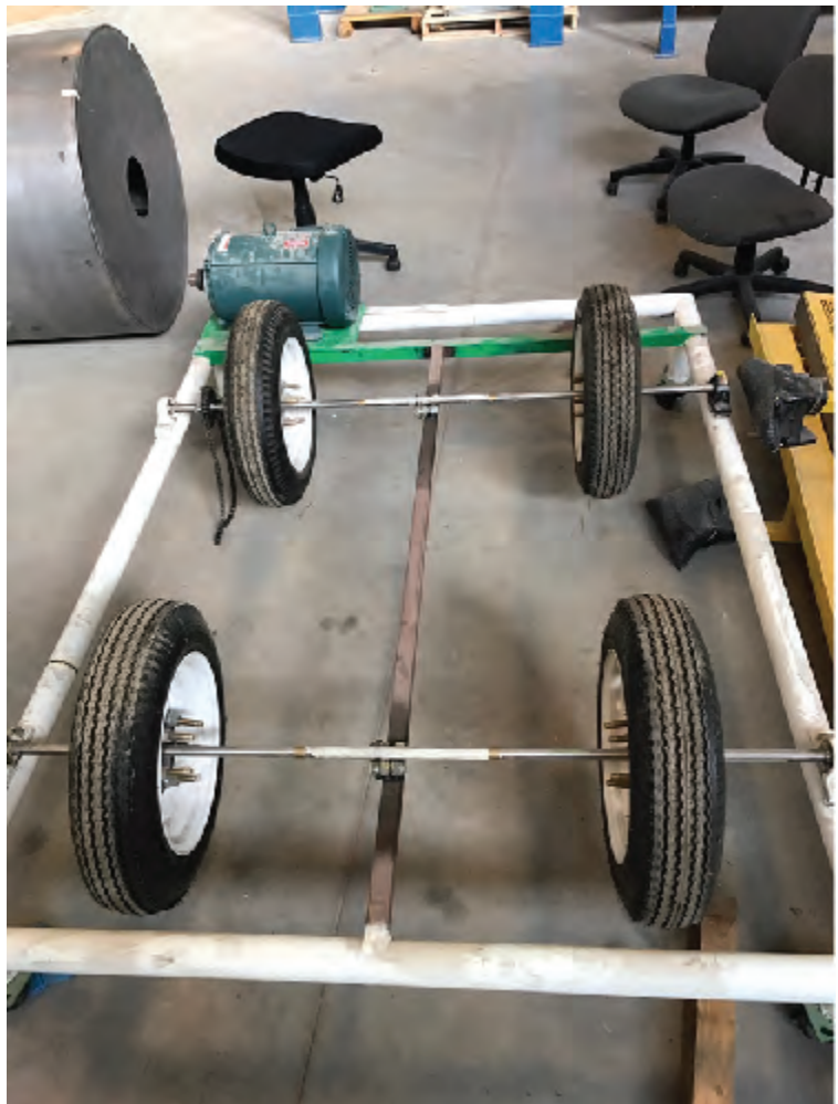
Figure 3 Base before adjustments with 7.5 HP motor at the back
