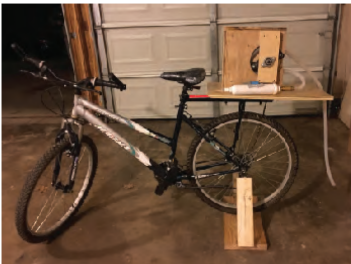
Figure 3 shows the bike stand which was built to hold the rear wheel and bike rack off the ground, allowing for stationary use.
